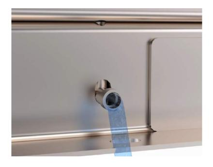
To properly engage to water management channel system the manhole frame has 25mm diameter outlet which must be connected to a positive drainage outlet pipe and not just a soakaway.
